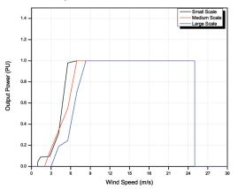
Fig. 21. Output Power Curve at different speed for small, medium and large scale wind turbine.
