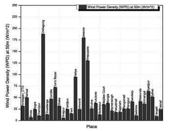
Fig. 13. Wind Power Density (WPD) at  $50m (W/m^2)$
