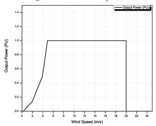
Fig 16. Output Power Curve at different speed for micro scale wind turbine.
