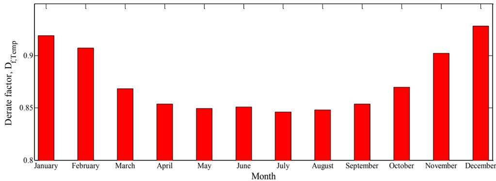
Figure 7. Variation in derating factor due to variation in the temperature.
