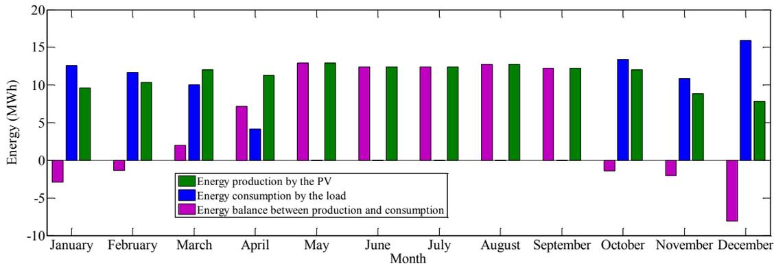
Figure 8. Energy performance of the designed PV system for the SQU sports complex.
