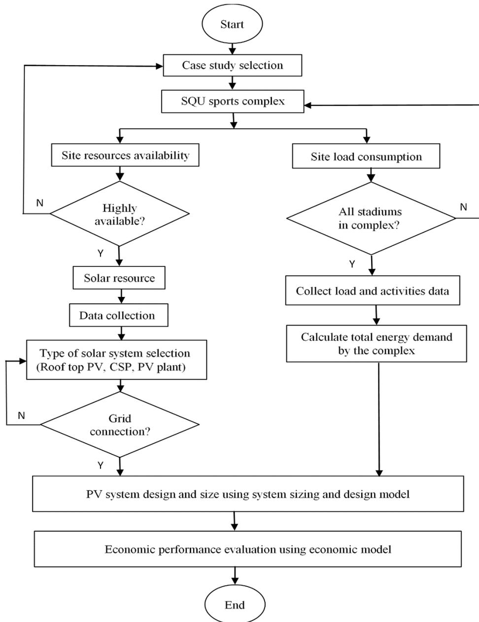
**Figure 6.** Flowchart of PV system design for SQU sports complex.
