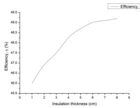
Fig. 5. Effect of insulation thickness on the system efficiency
