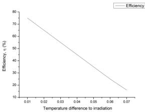
Fig. 9. Variation of efficiency with ratio of temperature difference to the solar radiation
