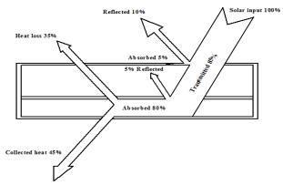
(Source: www.lth.se/fileadmin/ht/Kurser/MVK160/Project\_08/Fabio.pdf) Fig.1. Heat flow through a flat plate collecctor
