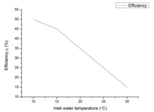
**Fig. 3**. Influence of the inlet water temperature on the system efficiency
