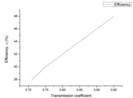
Fig. 7. Effect of transmission coefficient of the glass cover .
