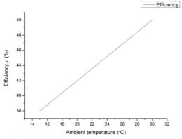
**Fig. 4.** Influence of ambient temperature on the system efficiency
