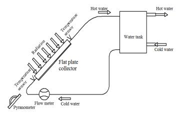
Fig. 2. Experimental setup
