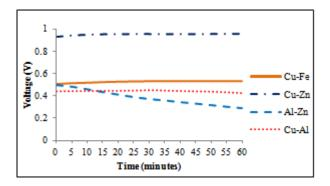
**Fig. 6.** Voltage profile over time obtained from banana tree (Musa acuminate) using different pairs of electrodes.
