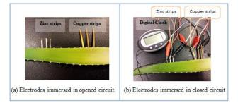
**Fig. 3.** Photos showing Aloe Vera with electrodes immersed in opened circuit and with closed circuit (connected with digital clock as load).
