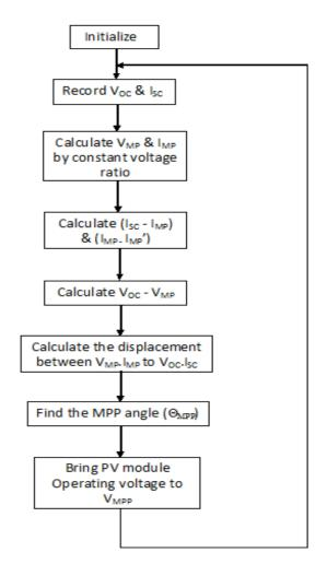
Fig. 7 Maximum Power Angle (MPA) algorithm
