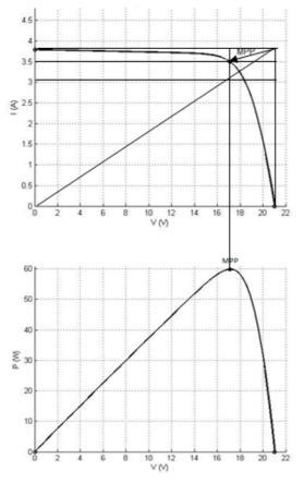
**Fig. 5.** Mechanism of maximum power point (MPP) angle method for MPPT
