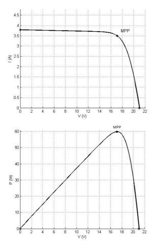
Fig. 4. Simulated I-V and P-V Characteristic Curves
