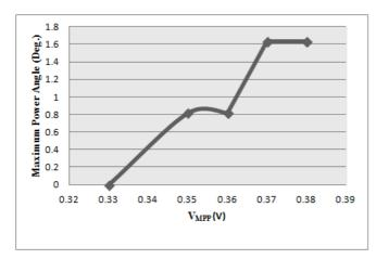
Fig. 8 Variation of maximum power angle with  $V_{MPP}$
