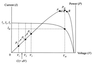
Fig. 1. Perturb and Observe (P&O) Technique for MPPT
