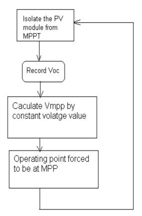
Fig. 3. Structure of Constant Voltage method
