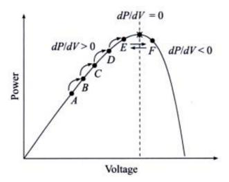
Fig. 2. Incremental conductance method for MPPT
