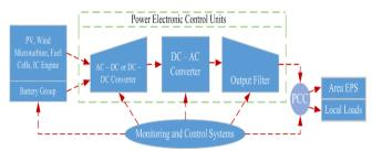
Fig.2. Power electronics of a typical DER system
