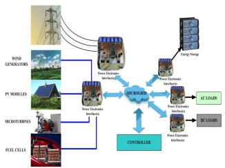
Fig. 3. Power electronics interface in a microgrid
