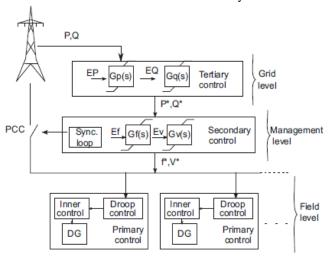
Fig. 4. Centralized hierarchical control of microgrids
