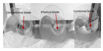
**Fig. 2.** Prototypes blade rotor conventional, elliptical and combined blade with end plates.
