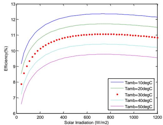
**Fig. 6.** Variation in Efficiency with solar irradiation
