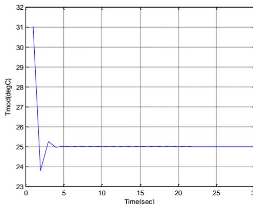
**Fig. 11.** Response of PI controller with reference temperature at 25°C
