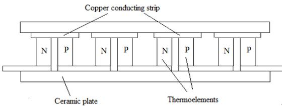
**Fig. 1.** Basic single stage thermoelectric module
