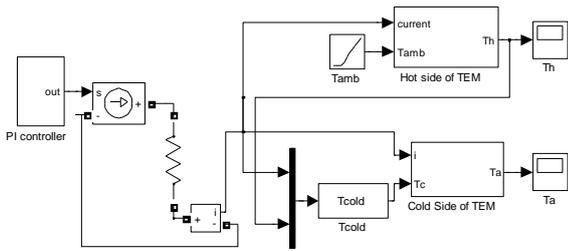
**Fig. 3.** Mathematical model of TEM developed for cooling mode
