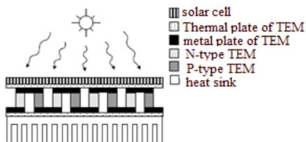
**Fig. 8.** PV cooling module with TEM attachment.
