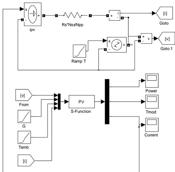
**Fig. 7.** Model of solar cell showing module temperature dependence on power output
