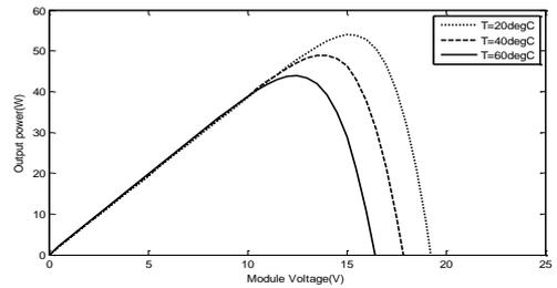
**Fig. 5.** Effect of PV module temperature on the output power
