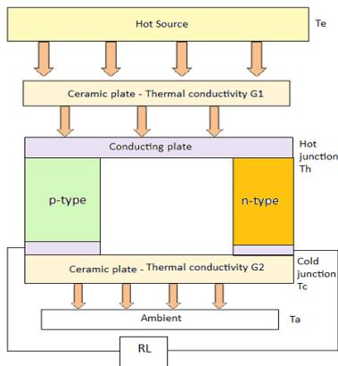
**Fig. 2.** A single thermoelectric couple used as Generator
