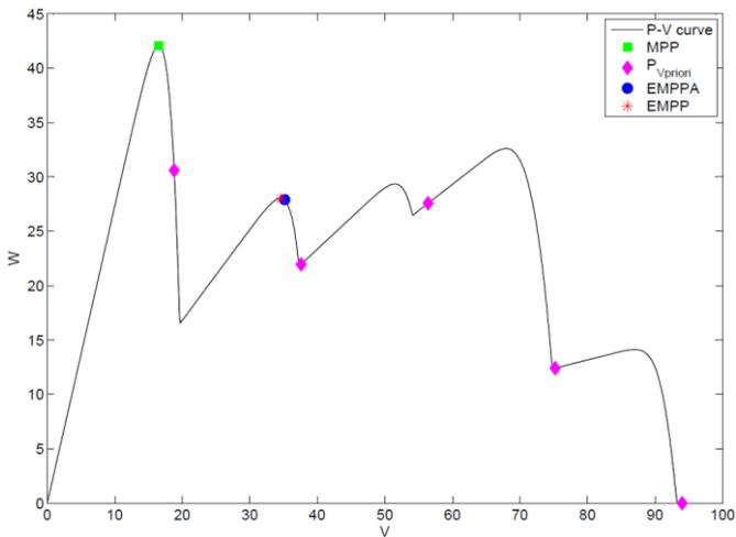
Fig. 3. The ANN fails in discovering the "hill" and the amount of wasted power is large.
