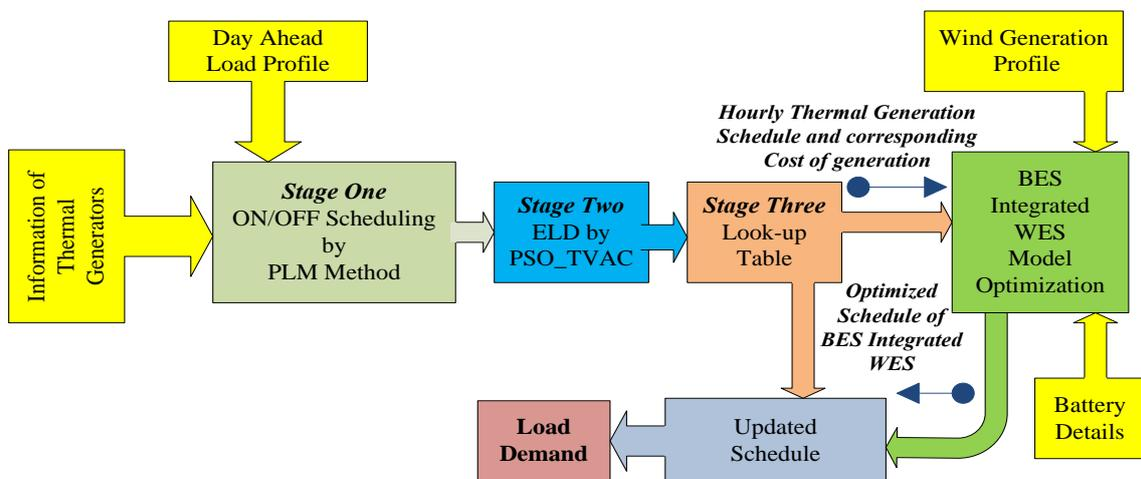
**Fig.1** Block Diagram representation of solution methodology
