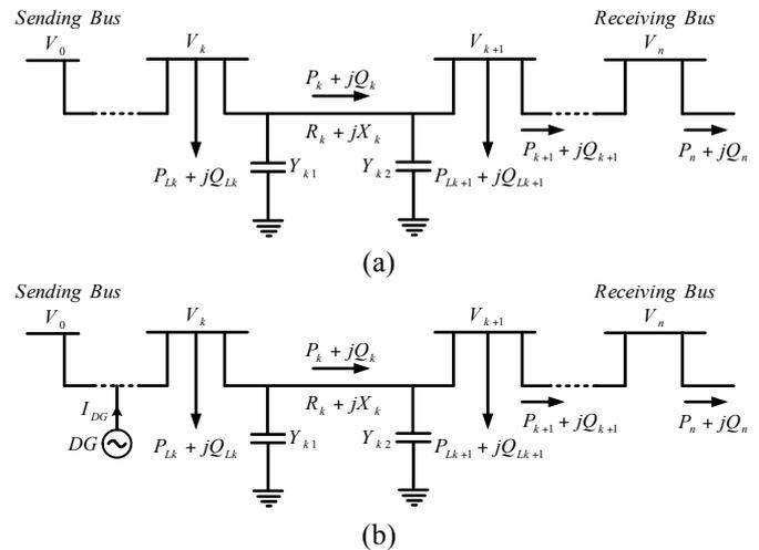
**Fig. 1.** A single-line diagram of a feeder (a) without DG (b) with DG
