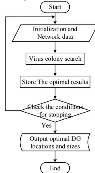
**Fig. 4.** The flowchart of searching for the optimal location of installation of the DG sources
