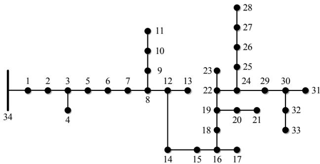
Fig. 5. The diagram of a single-line 34-bus IEEE standard system
