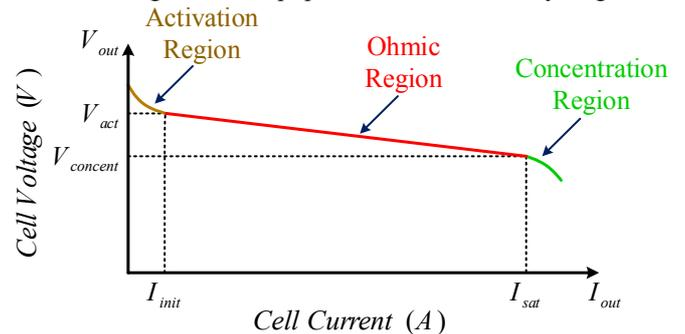
Fig. 2. The I-V curve of fuel cell
